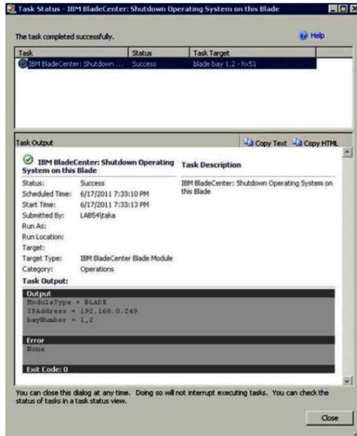
Figure 56. Task status indicating the shutdown task has been sent to this Blade
